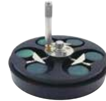
Sample Loading/Unloading Fixture (shown with 5-3461 sample holder)
